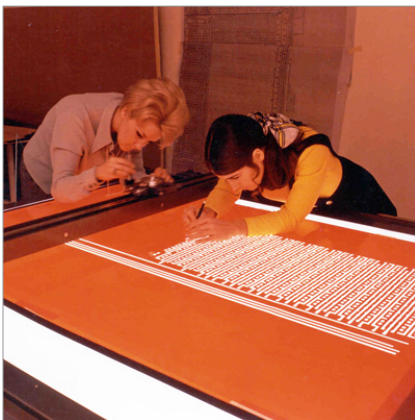
↑ Hand cutting an IC design onto rubylith material for creating the pattern to be optically shrunk onto a photographic mask – early 1970s
